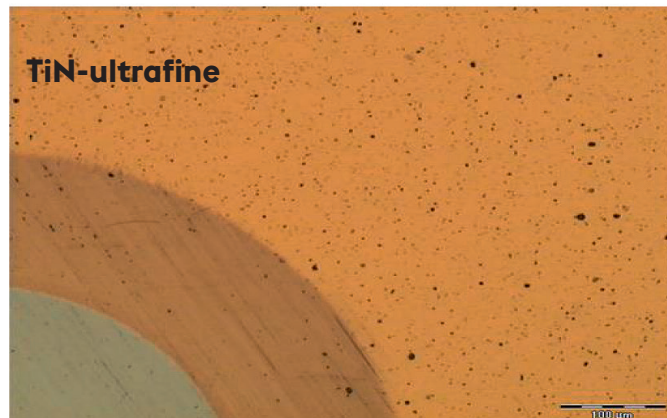
Fig. 1: Surface with calotte grinding of a standard TiN (top) and a TiN-ultrafine (bottom).
